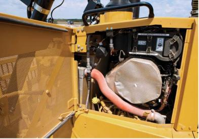
The D6T features a Cat C9.3 ACERT<sup>TM</sup> engine and a Cat Clean Emissions Module to deliver the performance and efficiency that customers demand, while meeting U.S. EPA Tier 4 Interim/EU Stage IIIB emission standards.
