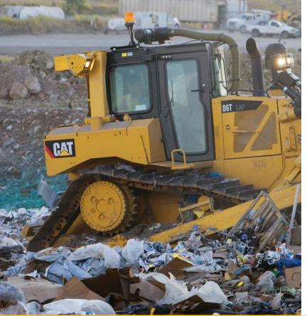
The D6T WH features the Cat elevated sprocket design that isolates final drives, axles, and steering components from harsh impacts. The undercarriage is designed for easy clean-out, and a modular design aids serviceability to help reduce maintenance costs.
